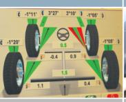
Imperfect alignment can result in irregular tyre wear and impaired handling. We take care of toe, camber and caster angle inspections using 3-D camera 4-wheel alignment technology at regular intervals.
